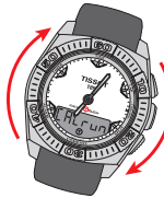
Turn the watch on itself for more than a complete revolution on a horizontal surface (e.g. a table) in an environment free from magnetic interference, at a rotation speed of around 30° per second. Total time: 20 seconds maximum
